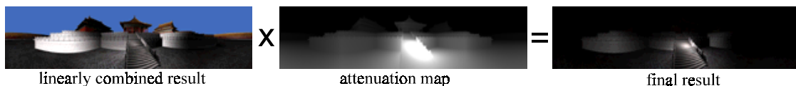
Figure 11. The distance fall-off effect can be simulated by multiplying the linearly combined result with an attenuation map.
