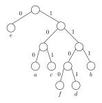
The depths of e, a, c, f, d, b are 1, 3, 3, 4, 4, 3, respectively. The average length of the encoding equals
