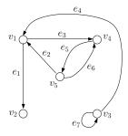
This is a directed graph (V, E) where there are 5 vertices  $v_1, v_2, ..., v_5$ , and 7 edges  $e_1, e_2, ..., e_7$ . Edge  $e_6$  is an outgoing edge of  $v_5$  and an incoming edge of  $v_4$ .
