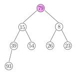
79 causes a violation by being greater than its children. This is fixed by swapping it with node 8, which is the child of the root with a smaller key. See the next slide.
