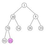
15 causes a **violation** by being smaller than its parent. This is fixed by a swap with its parent; see next.
