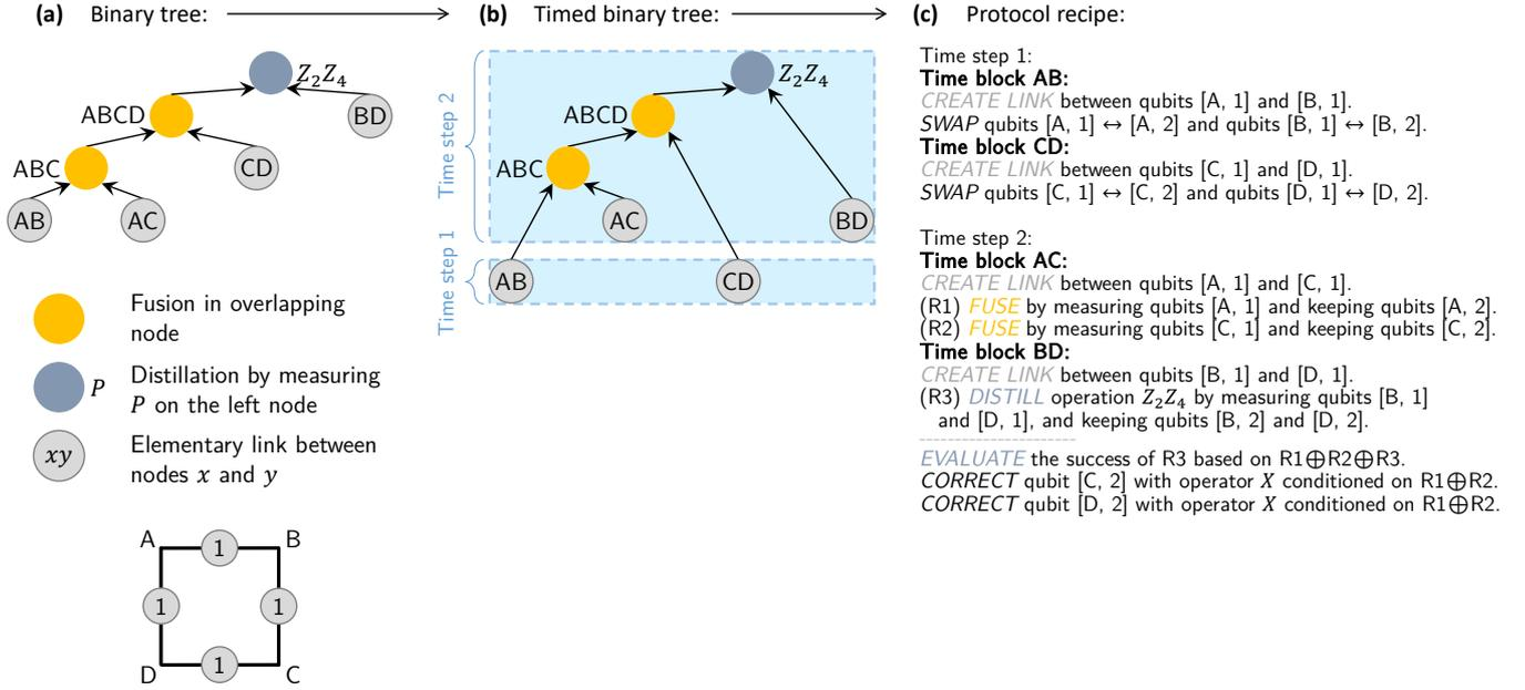
**Figure 1:** (a) Binary tree with  $K = 4$  found with the dynamic program of Ref. [2]. (b) Identified time steps for the operations in this binary tree. (c) Identified protocol recipe for this binary tree.
