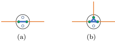
Figure 1: (a) A BSM measurement in the switch that fuses two quantum links by connecting two qubits. (b) A 3-GHZ measurement in a switch that fuses three quantum links by connecting three qubits. In both figures, the small blank circle in the switch denotes free qubits that are not entanglement, the small green circle in the switch denotes entangled qubits, the orange line indicates the quantum links to be fused, and the blue line shows the connection between qubits to fuse quantum links.
