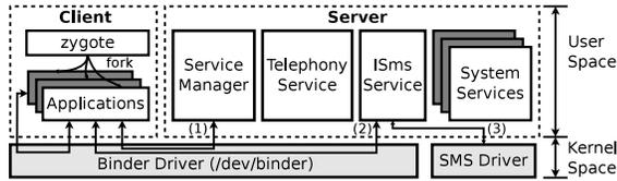
Figure 2: Binder IPC mechanism.
