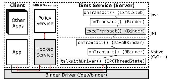
Figure 6: Call graph of ISms Binder transaction on the server side.
