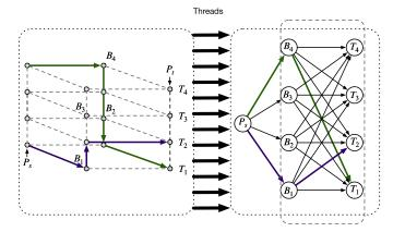
Fig. 8. GPU-friendly 3-D L-shape pattern routing; each 3-D L-shape pattern routing solution is denoted as  $\mathcal{P}\{P_s, B_{l_s}, T_{l_t}\}$ . There are two sample paths colored by green and purple.
