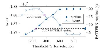
Fig. 12. Performance with different  $t_2$  for the design 18test5m, where  $t_1$  is 100; the solid circle line represents PATTERN runtime while the other is the global routing score. The *thick dashed line* is the baseline PATTERN runtime of CUGR and the other is the baseline score.
