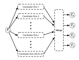
Fig. 10. Overall GPU-friendly 3-D Z-shape pattern routing flow.
