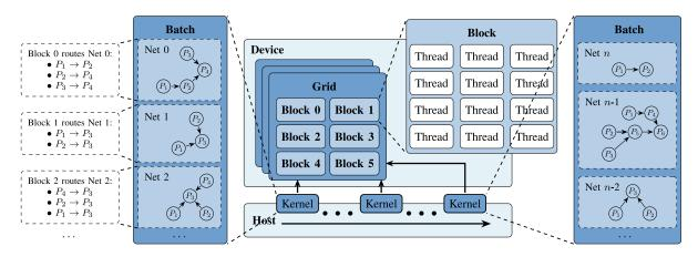
Fig. 7. Programming architecture for the pattern routing stage; on the host, the kernels are invoked sequentially and each of them is used to process a single batch of nets. The nets in the same batch will be routed simultaneously on different blocks on the device.
