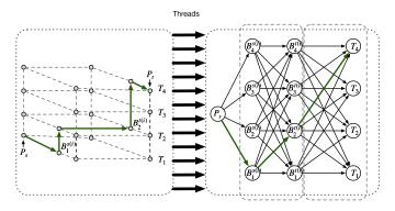
Fig. 9. GPU-friendly 3-D Z-shape pattern routing flow for *i*th candidate bend point pair  $(B^{s(i)}, B^{t(i)})$ ; each 3-D Z-shape pattern routing solution is denoted as  $\mathcal{P}\{P_s, B_{l_s}^{s(i)}, B_{l_t}^{t(i)}, T_{l_t}\}$ . The sample routing path is colored by green.
