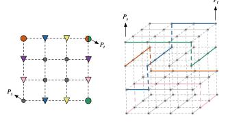
Fig. 11. Hybrid shape pattern routing; The left part shows all the bend point pairs and the right part contains four candidate 3-D solutions.
