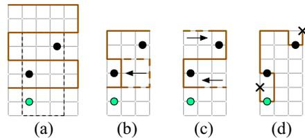
Fig. 11. Example of optimization for guidelines: (a) extract minimum bounding box that covers all qubits in the net (vertically extend by one grid for different candidates), (b) shift vertical segments to remove redundant horizontal segments, and (c) shorten dangling ending segments. (d) Example of generated routing in front face from the guideline in (b).
