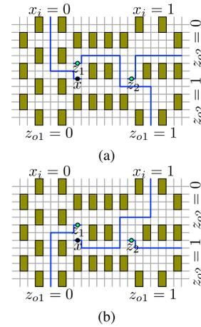
Fig. 18. Junction with two cases of input: (a)  $x_i = 0$  and (b)  $x_i = 1$ . Additional inverter is required for output  $z_{o1}$  at the bottom.
