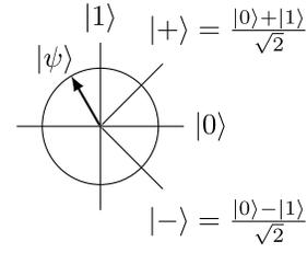
Fig. 2. Quantum state and different bases ( $|0\rangle$  and  $|1\rangle$  for Z-basis and  $|+\rangle$  and  $|-\rangle$  for X-basis).
