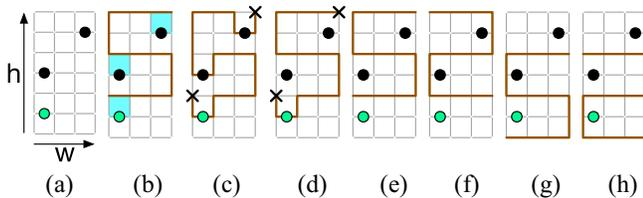
Fig. 10. (a) Example of net, where control qubit is marked by green dots and target qubits are marked by black dots and (b) a guideline for generating routing solution and (c) generated front face and (d) back face. Four possible guidelines for a net are shown in (e)–(h).
