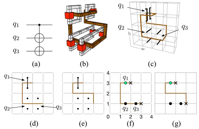
Fig. 7. (a) Example of a CNOT gate with two targets and (b) its implementation with one depth step and qubits placed in 2-D space and (c) corresponding 3-D stick diagram and (d) its front view and (e) its back view. Corresponding stick diagram: (f) front face and (g) back face.
