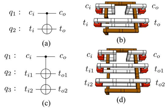
Fig. 4. (a) CNOT gate with  $q_1$  as control qubit and  $q_2$  as target qubit. (b) Primal-primal implementation of CNOT gate, where dual defects (brown) braid around primal defects (white) and red cubes represent inputs and outputs [8]. (c) Multiple-target CNOT gate with  $q_1$  as control qubit and  $q_2$  and  $q_3$  as target qubits. (d) Geometric description of the multiple-target CNOT gate.
