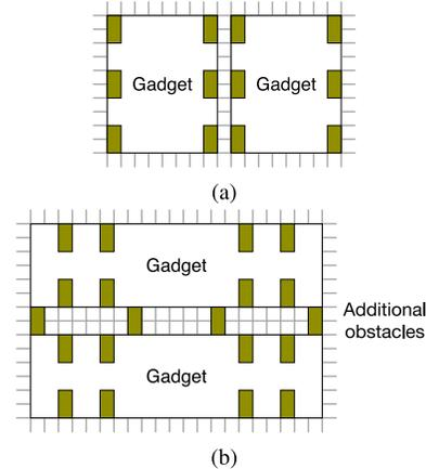
Fig. 20. (a) Horizontal and (b) vertical connection of gadgets. four additional obstacles are required for vertical connection.
