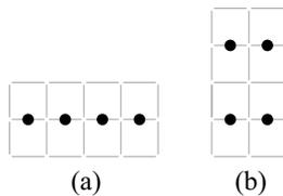
Fig. 8. (a) Example of single-layer qubit arrangement like that in Fig. 5(b) (view from left). (b) Two-layer qubit arrangement like that in Fig. 5(c).
