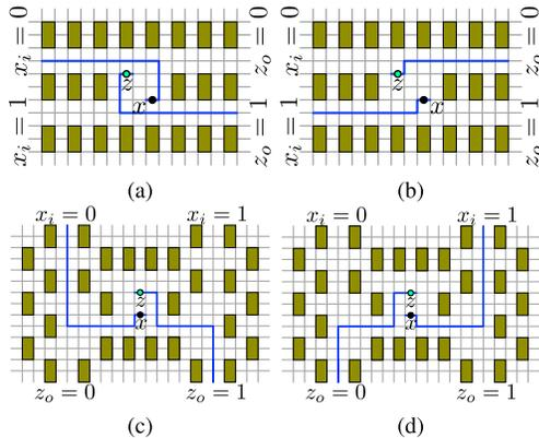
Fig. 17. Inverters with two cases of input: horizontal inverter (a)  $x_i = 0$ , (b)  $x_i = 1$  and vertical inverter (c)  $x_i = 0$ , (d)  $x_i = 1$ . Sources are in light green and sinks are in black, same for other figures in this section.
