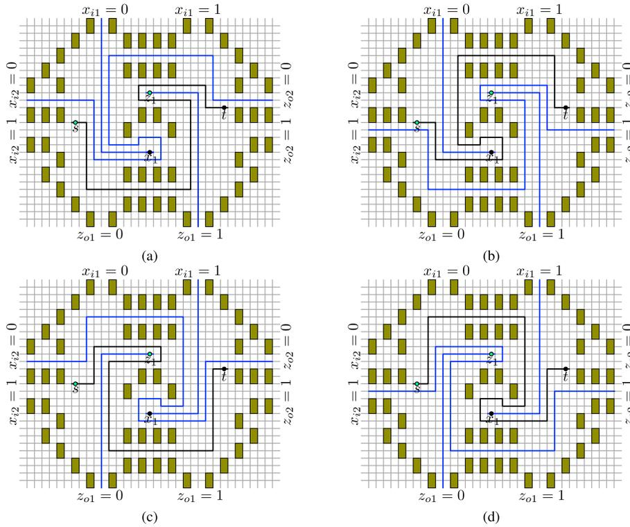
Fig. 21. Crossover with four cases of input:  $(x_{i1}, x_{i2}) =$  (a) 00, (b) 01, (c) 10, and (d) 11. Additional inverter is required for output  $z_{o1}$  at the bottom.
