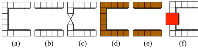
Fig. 3. Geometric components for measurement and initialization qubits. White cuboids denote primal defects and brown cuboids denote dual defects. (a) and (e) Z-basis measurement and  $|0\rangle$  initialization. (b) and (d) X-basis measurement and  $|+\rangle$  initialization. (c) State injection for  $|A\rangle$  or  $|Y\rangle$  initialization. (f) Generalized pin representation for primal defects, where the red cube generalizes the operation of initialization or measurement [6].
