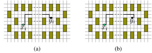
Fig. 13. Gadget to represent truth or false assignment of a variable. Example of (a) front path and (b) back path. The green rectangles denote obstacles. The source pin is marked light green and sink pin is marked black. The front path and back path are connected through their ending pins.
