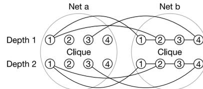
Fig. 12. Example of conflict graph for candidate routing solution assignment. The vertices within each gray circle form a clique and the connections are not drawn for brevity.
