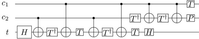
Fig. 6. Example of Toffoli gate implemented by a sequence of CNOT,  $T$ ,  $T^\dagger$ ,  $P$ , and  $H$  gates [32]. Its TQEC implementation, where  $T$ ,  $T^\dagger$ ,  $P$ , and  $H$  gates are implemented using teleportations can be seen in [6, Fig. 20].
