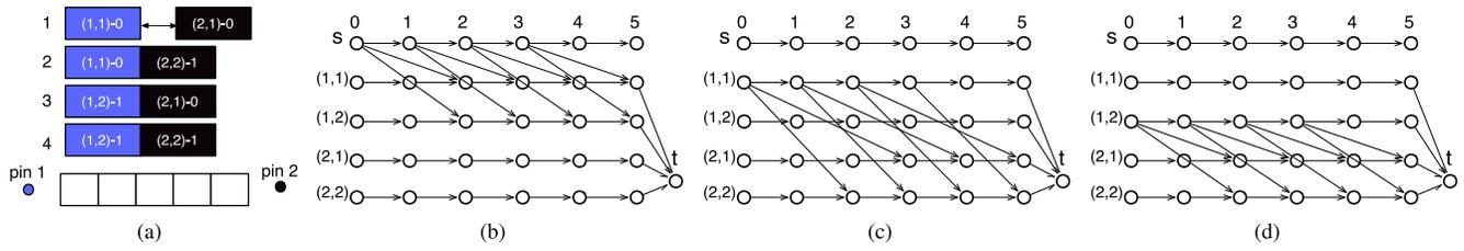
Fig. 9. Example for the TPL-OSR problem. (a) Two cells with different coloring solutions to be placed into a five sites row. Graph models with diagonal edges (b) from  $s$  vertex to first cell, (c) from  $c_{1_1}$  to second cell, and (d) from  $c_{1_2}$  to second cell.
