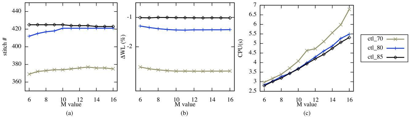
Fig. 14. TPLPlacer-MDP performance analyzes with different  $M$  values for alu design cases. (a) Impact on stitch numbers. (b) Impact on wire-length improvements ( $\Delta WL$ ). (c) Impact on runtimes.
