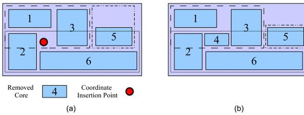
**Fig. 6** Clustering of cores during floorplanning. (a) The best candidate insertion point for the removed core  $c_4$ . (b) Update the floorplan result and bounding resources for clusters after insertion of the removed core  $c_4$ .
