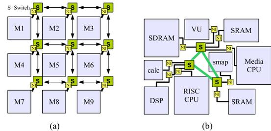
**Fig. 1** Two types of NoCs. (a) Regular NoCs. (b) Application-specific NoCs.
