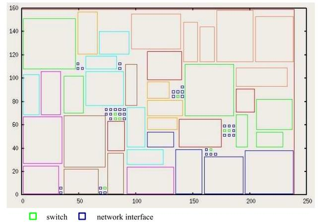
**Fig. 10** Floorplan of D\_38\_tvopd with switches and network interfaces.
