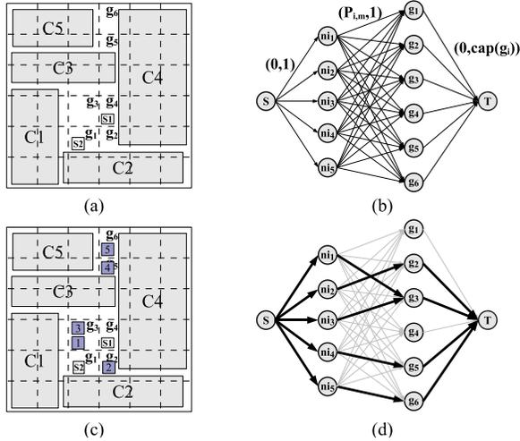
**Fig. 8** A sample of NIs insertion. (a) The candidate grids (*GRIDS*) for NIs insertion are the grids  $g_1, g_2, g_3, g_4, g_5, g_6$ . (b) Corresponding network flow model. (c) After min-cost max-flow algorithm, NIs insert into grids 3, 2, 3, 5, 6 respectively. (d) Corresponding network flow result.
