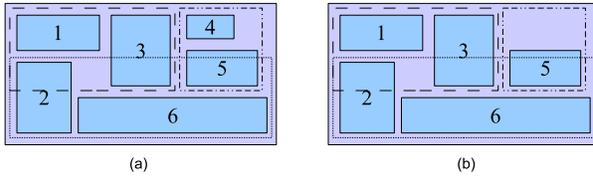
**Fig. 4** Floorplan and clustering of cores. (a) Initial floorplan and partition for the cores. (b) Floorplan and bounding resources for clusters after core  $c_4$  is removed.
