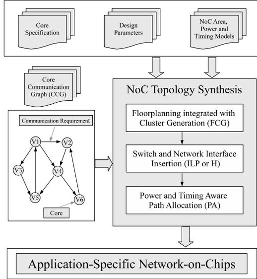
Fig. 2 NoC Design Approach Overall
