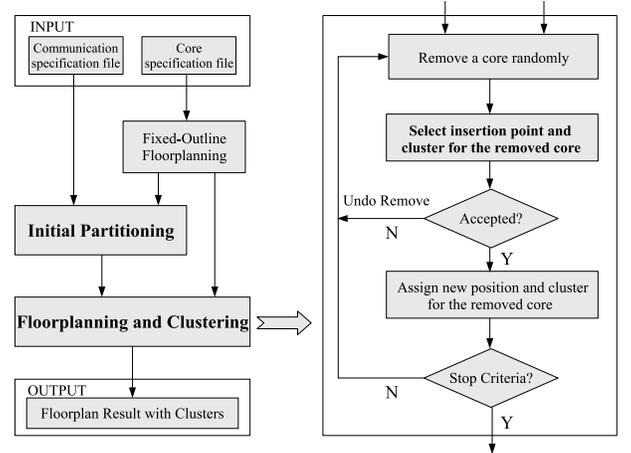
Fig. 3 Floorplanning integrated with Cluster Generation (FCG)
