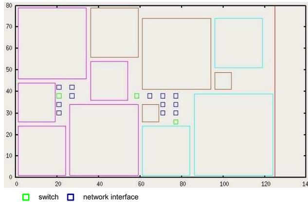
**Fig. 9** Floorplan of MPEG4 with switches and network interfaces.
