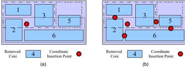
**Fig. 5** Candidate insertion points calculation. (a) Candidate cluster calculation for the insertion point. (b) Fixed number of candidate insertion points.
