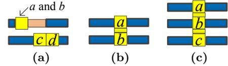
**Figure 2:** Different types of merging. (a) Merging on the same track.  $a$  is merged with  $b$ .  $c$  is merged with  $d$ . (b) Cuts  $a$  and  $b$  on adjacent tracks are merged. (c) Cuts  $a$  and  $c$  on non-adjacent tracks are merged. In such case,  $a$ ,  $b$  and  $c$  should be vertically aligned.
