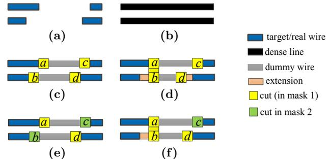
**Figure 1:** (a) A 1D target layout. (b) Dense lines. (c) Cuts and dummy wires. (d) The cuts are redistributed. (e) The cuts are assigned to different masks. (f) Incorporating cut redistribution with cut mask assignment.
