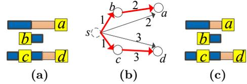
Figure 8: Illustration for the longest-path-based extension reduction method. (a) A cut redistribution and coloring solution, where the x-coordinates for  $a$ ,  $b$ ,  $c$  and  $d$  are 4, 1, 1 and 4, respectively. (b) The left-compactation graph and the longest paths. (c) The cut distribution after left-compactation.
