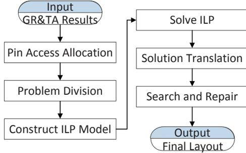
Figure 4: Overall flow of RVI enhanced detailed router
