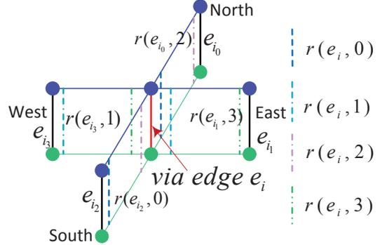
**Figure 3:** Direction-based redundant via variable.
