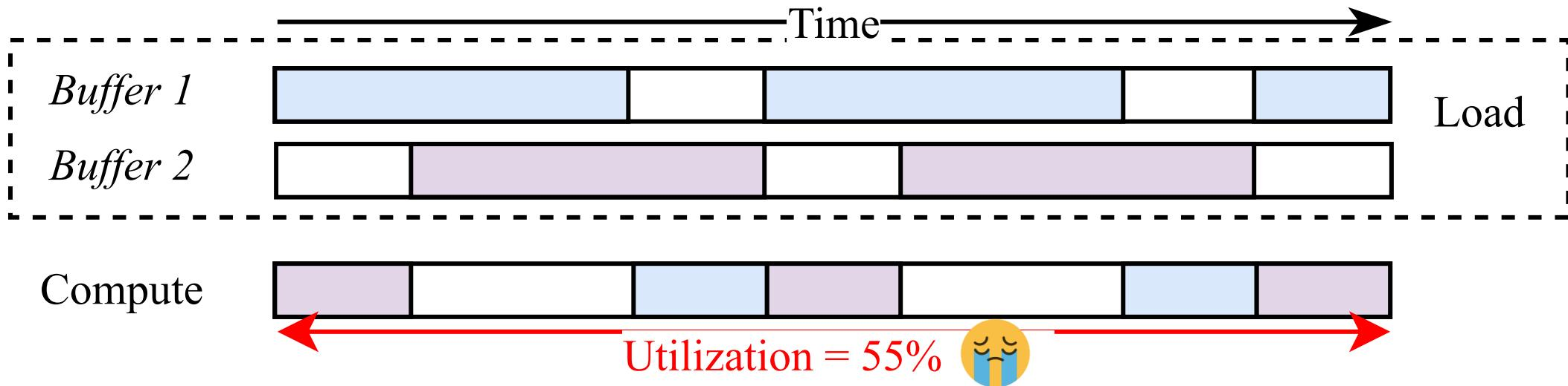
Limited number of stages (e.g. double-buffering) cannot fully hide the memory latency.
