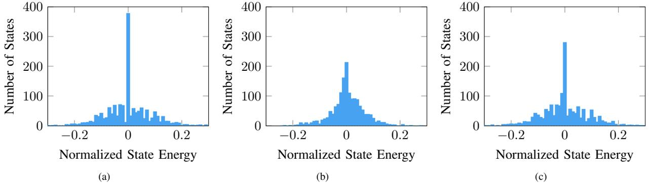
Fig. 2 Neighbor solution distribution for (a) area minimization; (b) wirelength minimization; (c) area and wirelength minimization.
