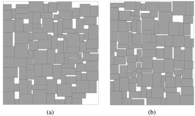
Fig. 4 Floorplan visualizations of the n100 netlist of GCRS benchmark: (a) n100 floorplan by simulated annealing; (b) n100 floorplan by our agent. The dead space of the floorplan by our agent is lower (7.95%) compared to that (8.88%) by Simulated Annealing.
