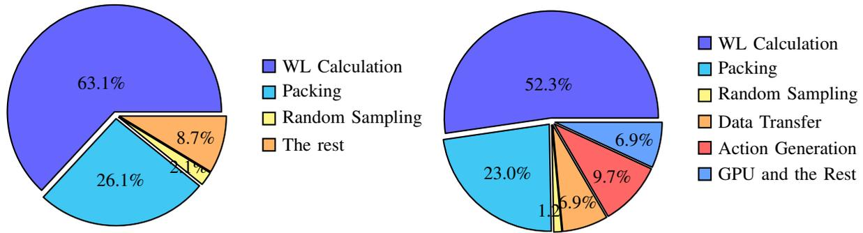
Fig. 5 Runtime profiling of the Simulated Annealing algorithm (left) and our agent (right). Most of the runtime (89.2% and 75.3%, respectively) is spent on solution evaluation (wirelength calculation and packing).
