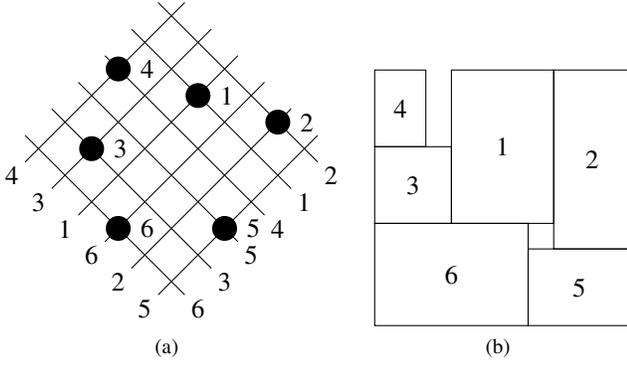
Fig. 1 (a) The oblique grid [25] shows the relative position between blocks for sequence pair  $\langle \langle 4\ 3\ 1\ 6\ 2\ 5 \rangle, \langle 6\ 3\ 5\ 4\ 1\ 2 \rangle \rangle$ ; (b) The corresponding packing. The dimensions for the 6 blocks are: 1( $4 \times 6$ ), 2( $3 \times 7$ ), 3( $3 \times 3$ ), 4( $2 \times 3$ ), 5( $4 \times 3$ ), 6( $6 \times 4$ ).
