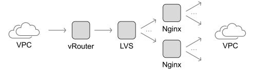
(c) Load Balancing. The traffic from the source VPC is routed to the destination VPC by vRouter, which then goes through two VGWs for load balancing. The LVS (Linux Virtual Server) balances Layer 4's traffic, while Nginx does Layer 7's.
