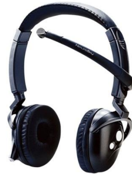
Figure 1.2-3 Wireless with a dry sensor - NeuroSky Mindset
