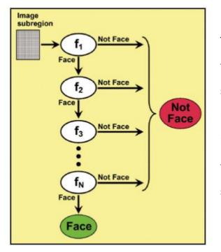
The word "cascade" means that the resultant classifier consists of several classifiers stages that are used subsequently to the interested region until at the stage that the case is rejected or all the stages are passed successfully.
