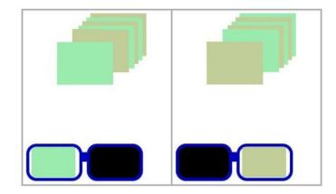
Figure 4.3 Principle of stereoscopy with active glasses
