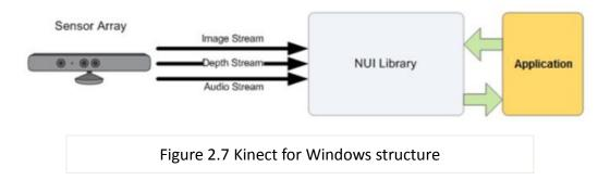
The SDK gives software library to help developers use the form of Kinect-based input like image, depth and audio. The Kinect and the software library interact with the application.
