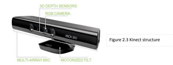
Kinect device have RGB camera, 3D depth sensor and multi-array microphone with a motorized pivot at the base. Using the Kinect, full body 3D motion could be captured. Apart from this, it could also recognize the face and voice.
