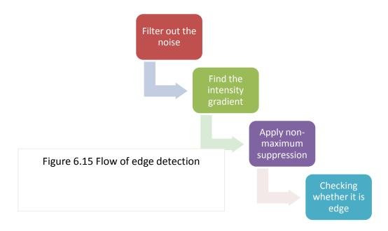
The Canny edge detector use the upper and lower thresholods for checking the edge of the image. If the pixel gradient is larger than the upper threshold, the piexl is meant to be edge. Meanwhile, if the pixel gradient is smaller than the lower, it is not edge. If the pixel garident is between the upper and lower thresholds, it would be edge if the connected pixel is larger the upper thresholds.
