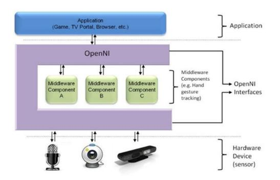
Figure 3.1 Three-layered view of the OpenNI Concept
