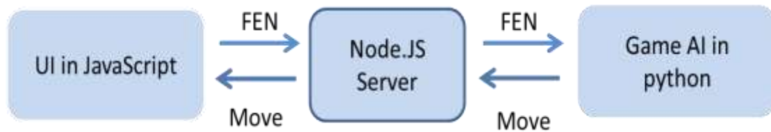
Figure 4.15. The Connection between Frontend and Backend
