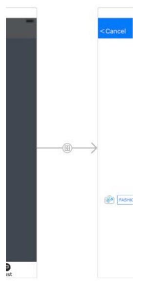
A segue in swift is for view transection. It controls how a user can go from one view to another view. In swift, it can be setup by just click and drag. It also allow programmer customizing his own segue. The default segue is not power enough for our use, so we have to implement the segue function by our own method instead of the given one.
