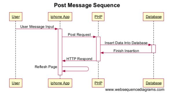
The above sequence diagram is show how the message being post to database. User input message and choose tag, after pressing the submit button, the app send a http post request with message information to the server, via the PHP a SQL insert command is send to database. Then the server will send back http respond to indicate the message is successfully upload. The app then refreshes the page to map view, the get message procedure will immediately invoked to update message information.
