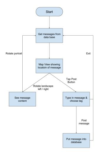
Mobile app may be suspended or interrupted by various event at any time, for example incoming phone, user pressing home button etc. In the above program flow diagram, the suspension and interruption problem is ignored. It only focuses on how the app works in foreground mode.
