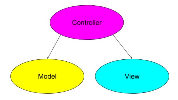
MVC is an object-oriented design pattern. Model object is defining the data and logic that manipulates that data. View object is presenting information and getting user input. Controller is performing set-up and coordinating tasks among model object and view object.
