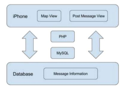
The above diagram is showing the server side system architecture. The iPhone application retrieves and uploads messages to database via PHP and MySQL. The data transfer is mainly the message content and message information.
