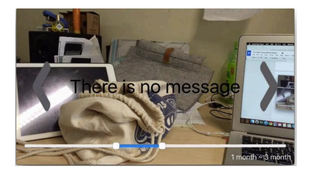
This is the second example. It shows that the user change the time interval, but still at the same position. The message checking view won't show the crying message. Instead of the crying message, it shows "There is no message" to indicate that there is no message in that particular time interval.
