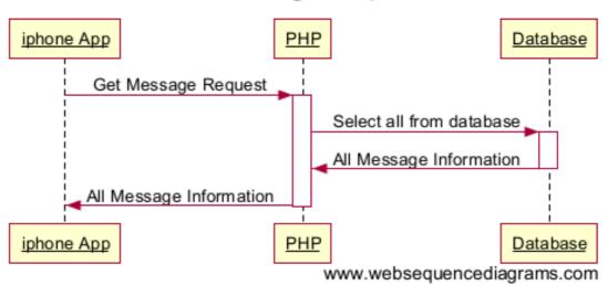
The above sequence diagram is showing how the message is get from the database. The app first sends a http request to server, via the PHP send a SQL command to database to retrieve all the message information. The messages will send back to app via the PHP by an http response. The above get message procedure will be invoked when map view is pull to the foreground.
