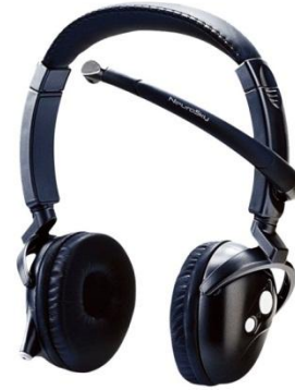
Figure 2-7 Wireless with a dry sensor - NeuroSky Mindset
