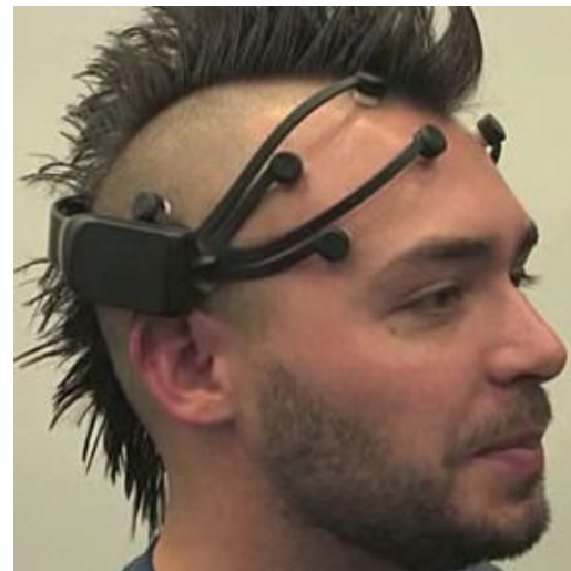
Figure 2-9 Highest number of sensors - Emotiv EPOC
