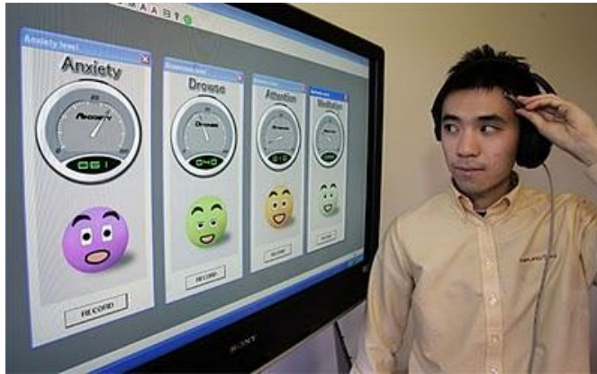
Figure 2-10 Some people find it difficult to establish perfect connection (Notice how the user holds the sensor closely towards the forehead)
