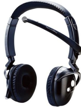
Figure 1.2-3 Wireless with a dry sensor - NeuroSky Mindset
