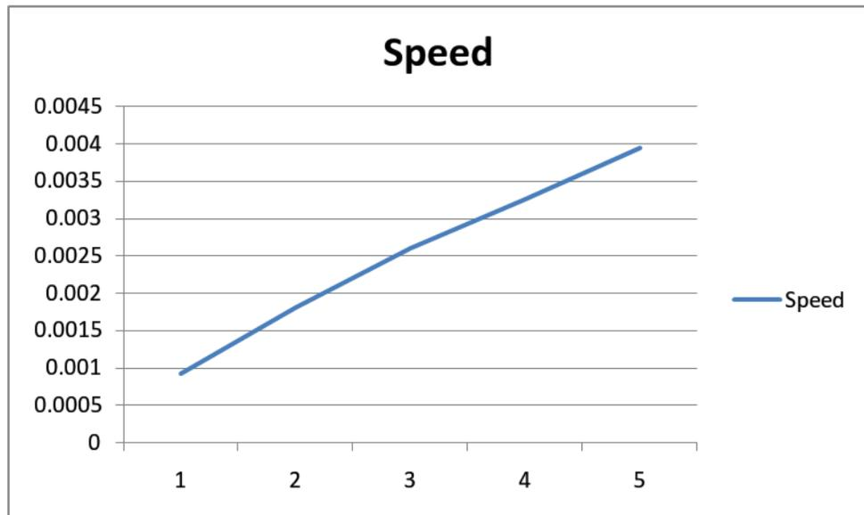
From the graph we see that speed is almost linear proportional to the number of nodes. This program tests on the I/O of HDFS, Job splitting, Shuffling and Sorting of Hadoop, the result shows that Hadoop is good on data processing.
