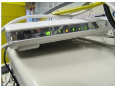
Most of the machines are connected to this switch in order to achieve 1000M bandwidth and eliminate the bottle neck of the network
