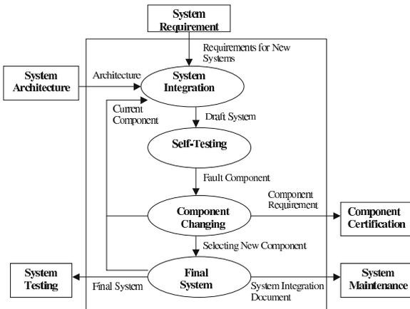
Fig. 9. System integration process overview.
