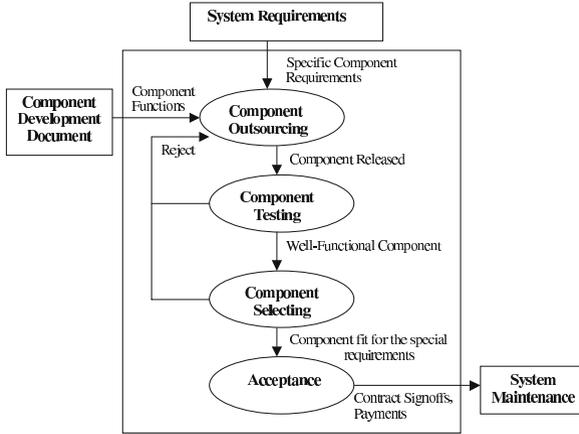
Fig. 6. Component certification process overview.
