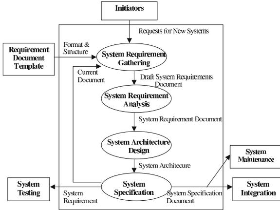
Fig. 8. System architecture design process overview.
