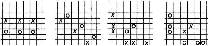
**Fig. 6.** Four configurations to extract features with  $\times$ 's and  $\circ$ 's representing black pixels and white pixels respectively. These configurations will be rotated clockwise with angles  $90^\circ$ ,  $180^\circ$  and  $270^\circ$ , respectively
