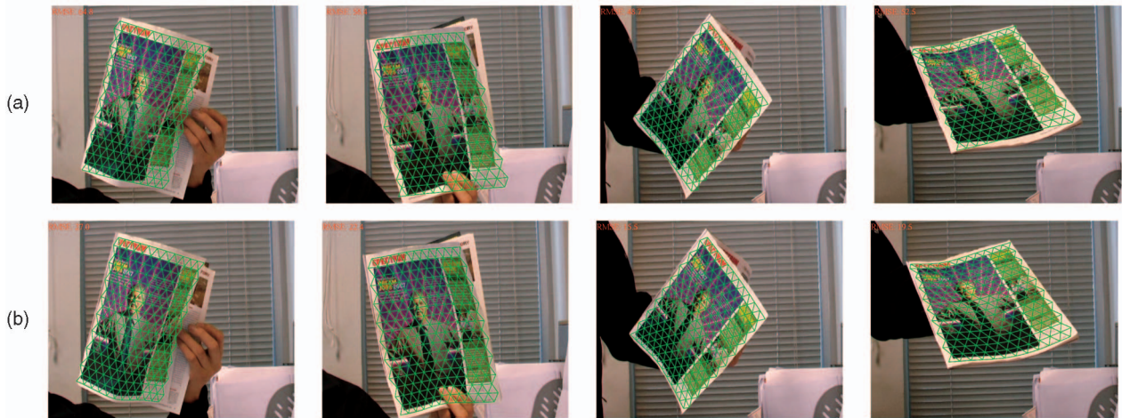
Fig. 18. Recovering the cover of a magazine in a real-time video with the size of 720 \times 576 . (a) shows the initialization results using feature correspondences only. (b) shows the results with the fusion approach. Moreover, the Root Mean Square Error (RMSE) is shown at the left corner in each image.
