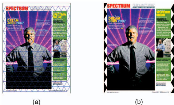
Fig. 2. (a) The mesh model with 216 vertices and 374 triangles. (b) The reference image size of 403 \times 516 . (a) Model mesh s_0 . (b) Reference image.
