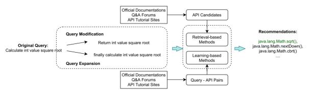
Fig. 1. The typical guery-based API recommendation framework.
