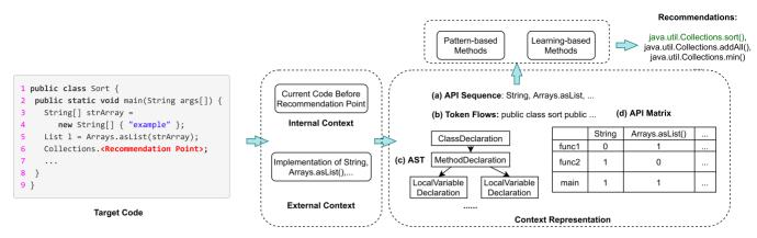
Fig. 2. The typical code-based API recommendation framework.
