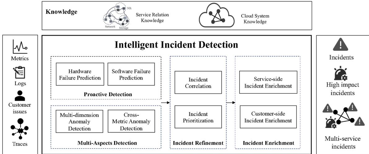
Figure 3. Intelligent incident detection framework.
