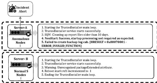
Figure 2. An incident example with relevant service-side console logs (shown in bold).
