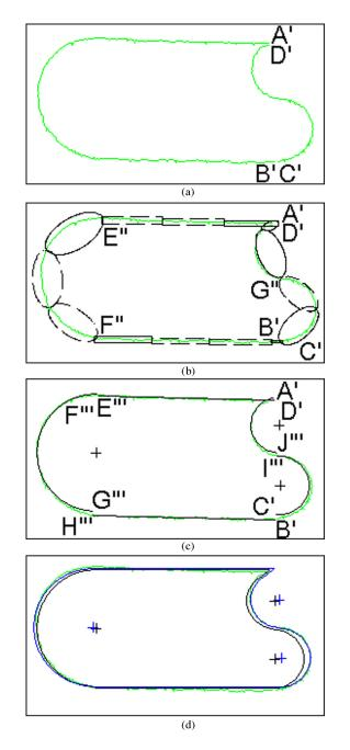
Fig. 1. Graphical primitives are extracted from a sketch. (a) A sketch with two strokes A'B' and C'D'. (b) Substrokes A'E'', E''F'', F''B' are extracted from stroke A'B' and C'G'' and G''D' are from C'D'. (c) Fitted results of substrokes are line segments A'E''' and H'''B' and arcs F'''G''', C'I''' and J'''D'. (d) Refined graphical primitives are label in black, and ground-truth ones manually extracted in blue. (Color version available online at http://ieeexplore.ieee.org.)
