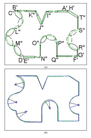
Fig. 4. Graphical primitives extracted from a sketch with part shape. (a) A sketch with four strokes A'B', C'D', E'F', G'H'. Substrokes A'I'', I''J'', J''K'', K''B' are extracted from stroke A'B', C'L'', L''M'', M''D' from C'D', E'N'', NO'', O''P'', P''Q'', Q''F' from E'F', and G'R'', R''S'', S''T'', T''H' from G'H'. (b) Refined, ground-truth graphical primitives of the sketch are labeled in black and blue, respectively. (Color version available online at http://ieeexplore.ieee.org.)
