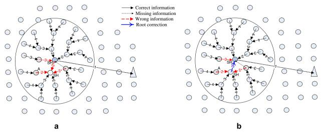
Fig. 5. Example of intruder identification with multiple malicious nodes.
