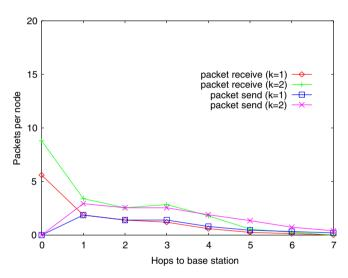
Fig. 15. Communication cost for intrusion detection.
