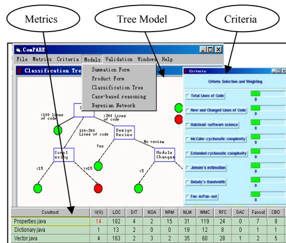
Figure 3. GUI of ComPARE for metrics, criteria and tree model
