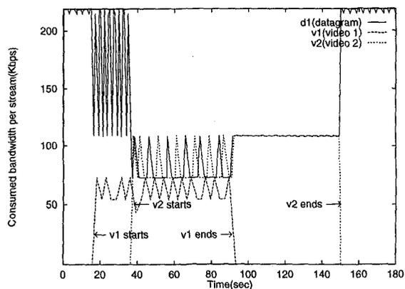
Fig. 3. Channel bandwidth usage, with QoS support disabled
