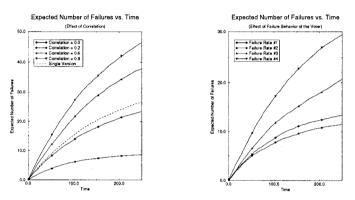
Figure 3. NVP - Failure Behavior in the Absence of Hardware Failures
