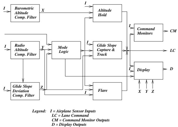
**Figure 4. Autoland system functions and data flow diagram**
