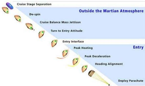
Figure 4. Procedures of landing system.
