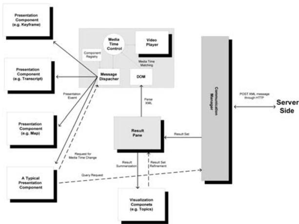
**Figure 9: iVIEW Visualization and Presentation Subsystem Architecture**
