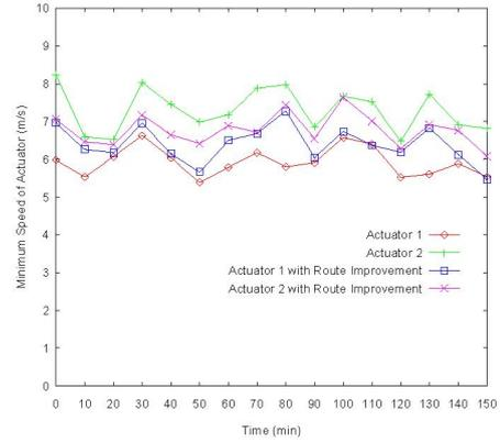
Figure 5. Speed of actuators with multi-route improvement.
