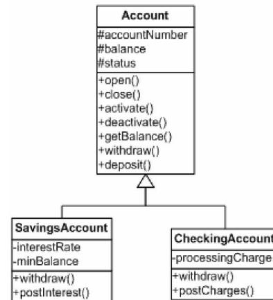
Fig. 3. Class diagram for Bank Account hierarchy
