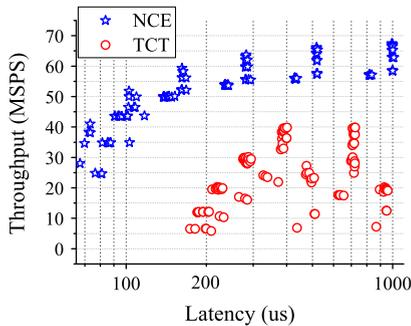
Fig. 7. Throughput and latency on 3M name table (average workload,  $\alpha = 0.5$ ).
