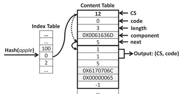
Fig. 4. Hash table data structure: component hash table.
