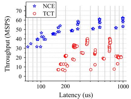
Fig. 10. Throughput and latency on 10M name table (heavy workload,  $\alpha = 0.5$ ).
