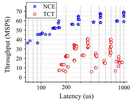
Fig. 9. Throughput and latency on 10M name table (average workload,  $\alpha = 0.5$ ).
