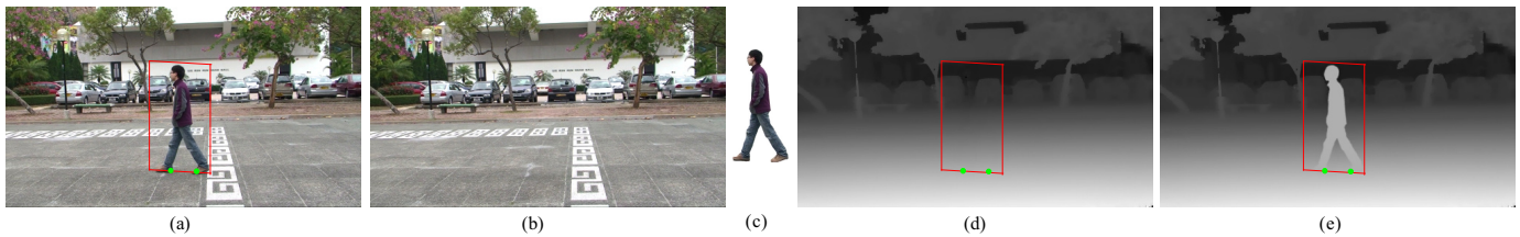
Fig. 6. Video sprite extraction with background completion. (a) One frame from an input video in which we want to extract the man. (b) The completed background by re-projecting pixels from other frames. (c) The extracted sprite. (d) The automatically computed background depth map. (e) To determine the position of the sprite plane, we only need two clicks at the contact points between the person and the ground.
