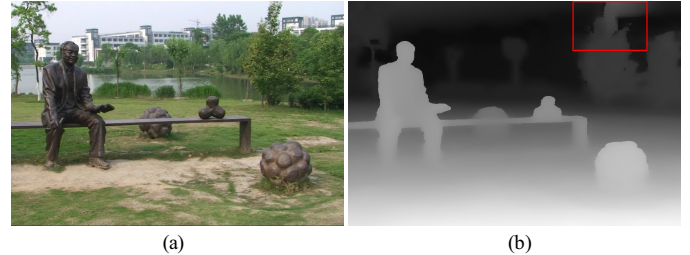
Fig. 16. A video frame (a) and the estimated depth map (b). In the red rectangle, because the disparities around the tree branches have inherent depth ambiguity regarding the nearly-constant-color background sky, the depth estimates are not all correct.
