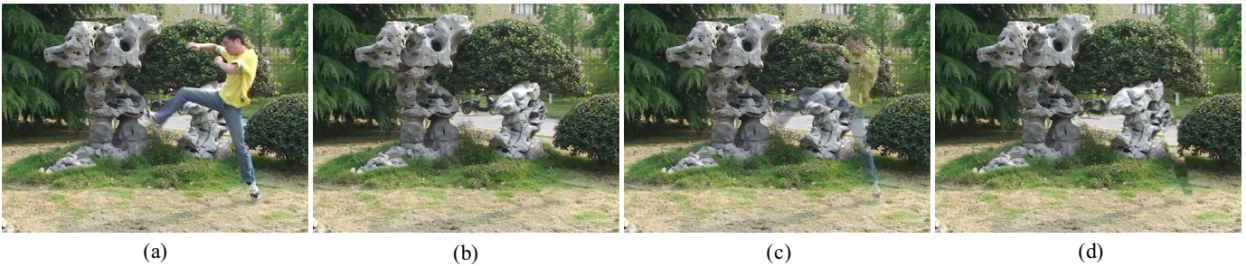
Fig. 13. “Predator” effect. (a) One original frame. (b) The recovered background image. (c) The actor becomes transparent. (d) The actor is camouflaged with the “predator” effect.
