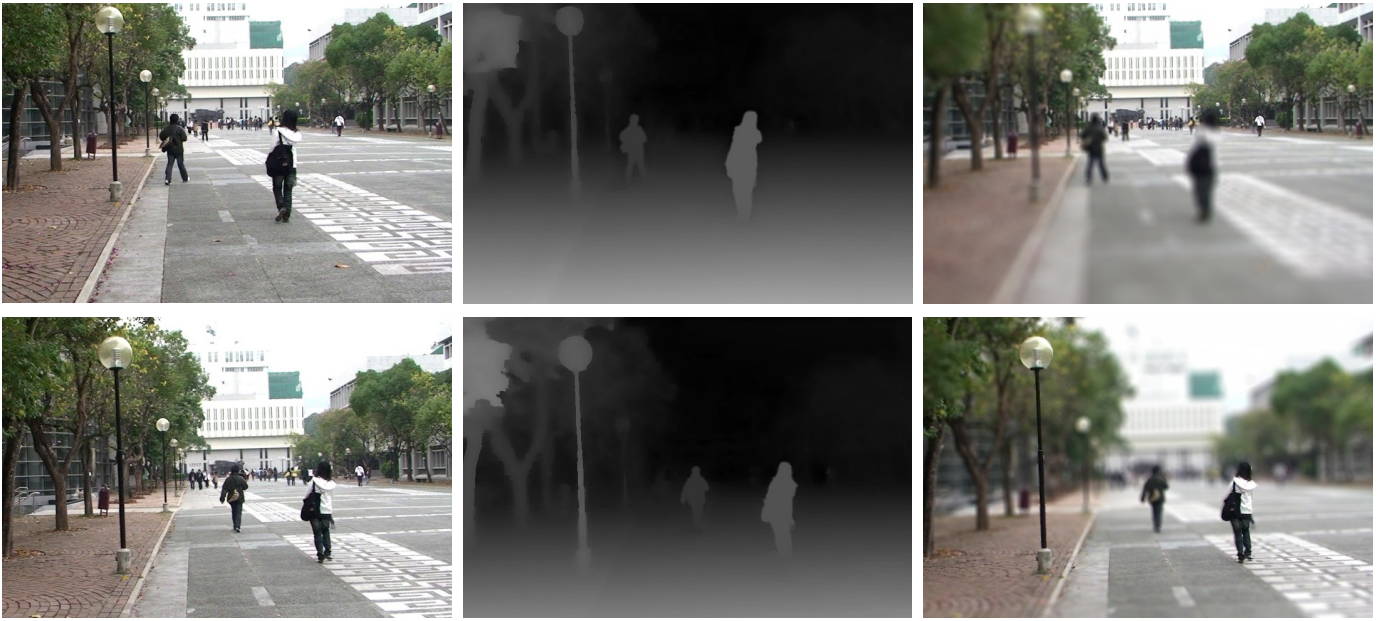
Fig. 12. Depth-of-field. The left-most column shows two frames from an input video. The middle column shows the recovered depth maps. The right-most column shows the result of changing the depth of field.
