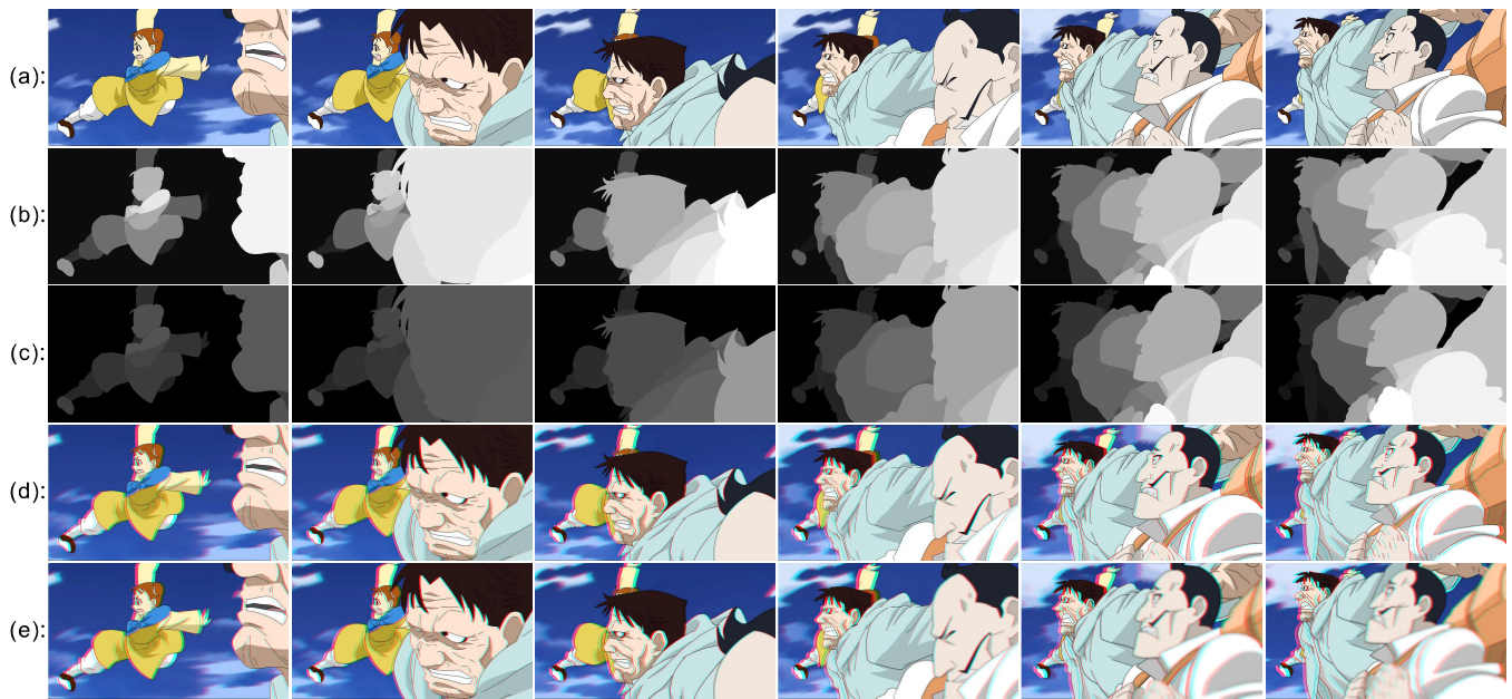
Figure 12: “Running.” (a) Input frames. (b) Topologically sorted ordering graph visualized as intensity. (c) Depth maps. (d) Stereo result. (e) Stereo result with out-of-focus effect. This sequence has 12 frames ( 1920 \times 1080 ). The frame containing the maximal number of regions has 72 regions. Depth ordering takes 13.5 minutes, and depth synthesis takes 10.9 minutes.
