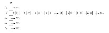
For this hash function, the maximum query time is the cost of scanning a linked list of 8 elements (i.e., the worst possible).
