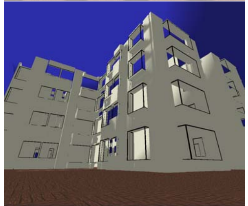
Figure 10: More challenging example. Top left: input floorplan, top right: preprocessed plan; middle: reconstructed interior model, bottom : exterior model obtained by specifying 4-storey building output.
