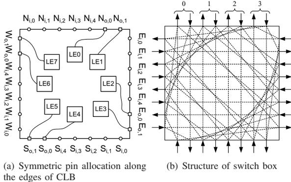
Fig. 2. Detailed FPGA fabrics for symmetric architecture
