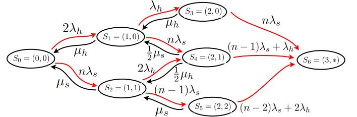
Fig. 3: State transition diagram of the Markov model for EPLOG's RAID-6.
