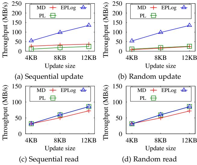
Fig. 6: Experiment S2: I/O performance measured by `fio` under 6+2-RAID-6 in normal mode (without any SSD failure).
