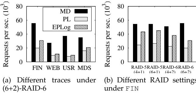
Fig. 10: Experiment S9: I/O performance comparisons under real-world traces
