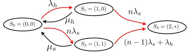
Fig. 2: State transition diagram of the Markov model for EPLOG's RAID-5.
