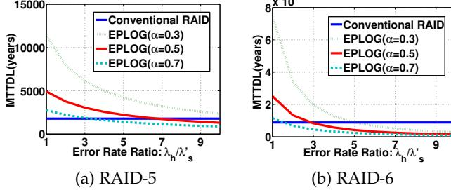
Fig. 4: Reliability comparison between EPLOG and conventional RAID.
