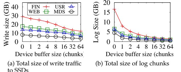
Fig. 5: Experiment S1: Impact of different device buffer sizes under (6+2)-RAID-6.
