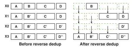
Fig. 2. Example of reverse deduplication for four backups of the same series created in the order X0, X1, X2, and X3.
