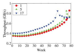
Fig. 9. Restore throughput of RevDedup with different live window lengths.
