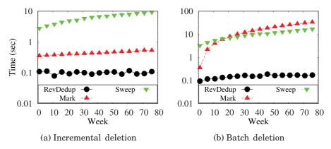
Fig. 10. Deletion times of RevDedup and mark-and-sweep.
