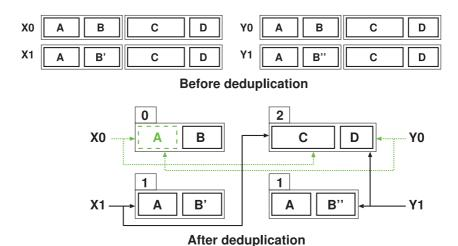
Fig. 3. Example of reference management in RevDedup for two backup series  $\{X0,X1\}$  and  $\{Y0,Y1\}$ , where X0 and Y0 are in the archival window, while X1 and Y1 are in the live window.
