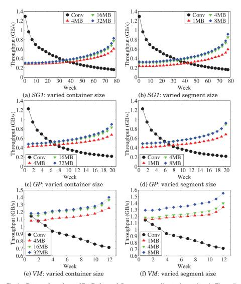
Fig. 6. Restore throughput of RevDedup and Conv, corresponding to the settings in Figure 5.
