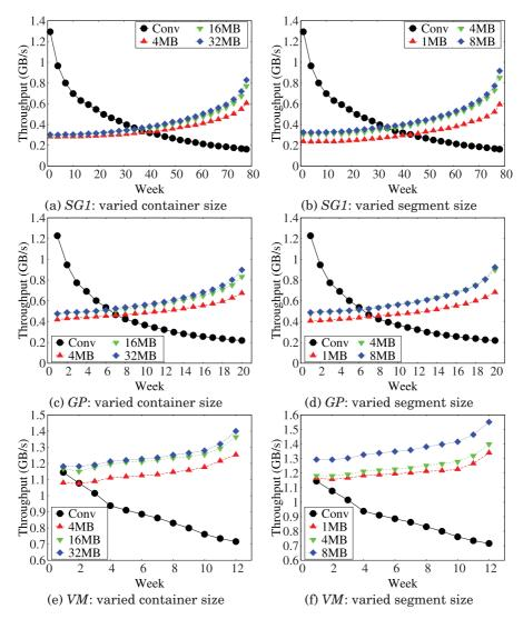
Fig. 5. Backup throughput of RevDedup and *Conv* for different datasets. We vary the container and segment sizes of RevDedup: (a), (c), and (e) fix the segment size at 4MB and vary the container size; (b), (d), and (f) fix the container size at 32MB and vary the segment size. The plots start from the second week to take into account interversion redundancy.
