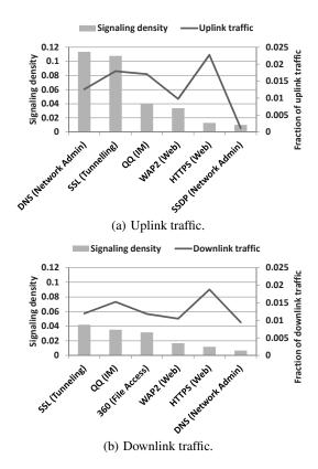
Figure 13: Breakdown of the state transitions triggered by uplink and downlink traffic for the top eight network applications.
