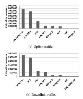
Figure 9: Distribution of signaling messages triggered by different types of TCP packets.
