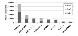
Figure 11: Breakdown of the state transitions triggered by top eight TCP packets without TCP payload (in descending order) that trigger the largest number of signaling messages.
