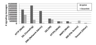
Figure 12: Signaling message distribution of the top eight network applications inducing the largest number of signaling messages (in descending order).
