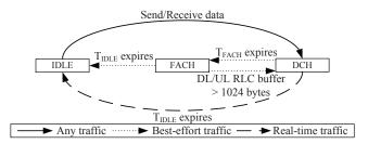
Figure 2: The RRC state machine for the UMTS network considered in this paper.
