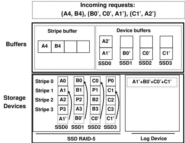
Fig. 3: Illustration of buffers in EPLOG.
