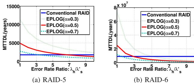
Fig. 6: Reliability comparison between EPLOG and conventional RAID.
