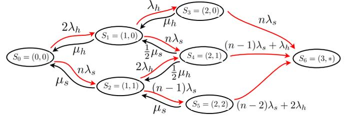
Fig. 5: State transition diagram of the Markov model for EPLOG's RAID-6.
