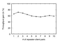
**Figure 15:** *Improvement in throughput with multiple repeater-client pairs.*
