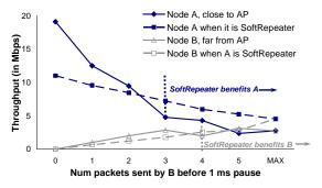
**Figure 12:** AP sends full blast traffic to A, and sends bursts of packets to B with a pause for 1 ms. MAX corresponds to back to back UDP packets.
