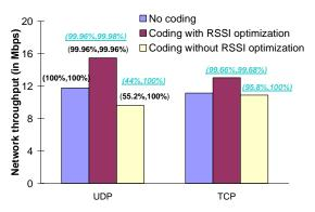
Figure 10: Throughput improvement due to network coding, and impact of RSSI optimization
