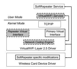
Figure 2: The SoftRepeater Architecture.
