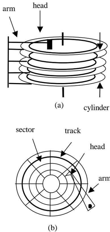
Fig. 1 Disk view (a)side view (b)top view
